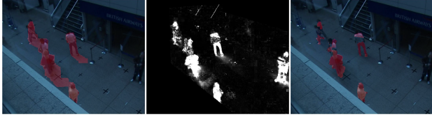
Figure 5: An Extreme FG/BG Segmentation Example : Here we show segmentation results for the foreground- (left) and background-biased (right) MRFs for frame 500 of clip S08 . The frame shown here is a somewhat extreme example of the different solutions found by the two MRFs. Both MRFs use the Mahalanobis distance values visualized in the middle image as the background label potential. For display purposes, the intensity is saturated at a distance of 64, twice the foreground potential for the background-biased MRF (so a 50% gray pixel sits on the classification threshold, absent any neighborhood effects).
