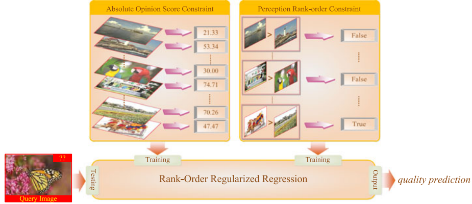
Fig. 1. Diagram of rank-order regularized regression. The absolute opinion score constraint drives the regression function to improve the prediction accuracy of each image. The perceptual rank-order constraint refines the regression function to improve the consistency of the quality rank-order of each pair of images.
