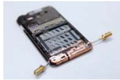
The prototype of testing CRDN in a smart phone with dual antennas
