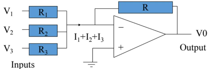
$$V_0 = -R \cdot \left\{ \frac{V_1}{R_1} + \frac{V_2}{R_2} + \frac{V_3}{R_3} \right\}$$
