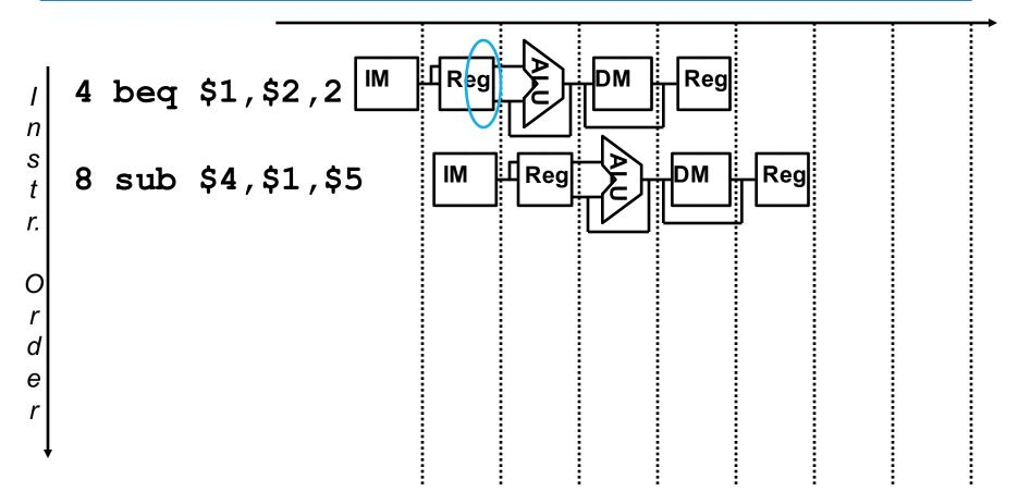
To flush the IF stage instruction, assert IF.Flush to zero the instruction field of the IF/ID pipeline register (transforming it into a nop)
