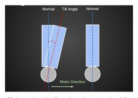
$\label{eq:motion} \mbox{Motion against the tilt angle, so it can stand upright.}$
