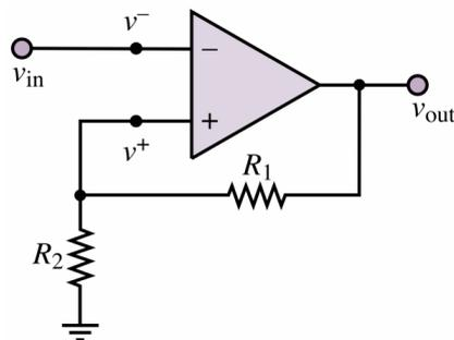
Figure 5: Schmitt Trigger
