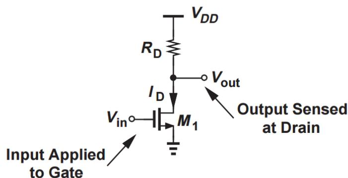
Figure 7: Common Source Amplifier
