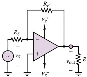
Figure 6: Inverting Amplifier
