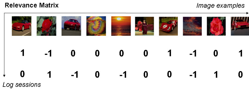
Figure 7.2: The relevance matrix for representing the log information of user feedback. Each column of the matrix represents an image example in the image database and each row of the matrix corresponds to a log session in the log database.
