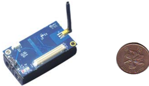
Figure 1.2: IRIS Mote: A typical low-end sensor node hardware platform
