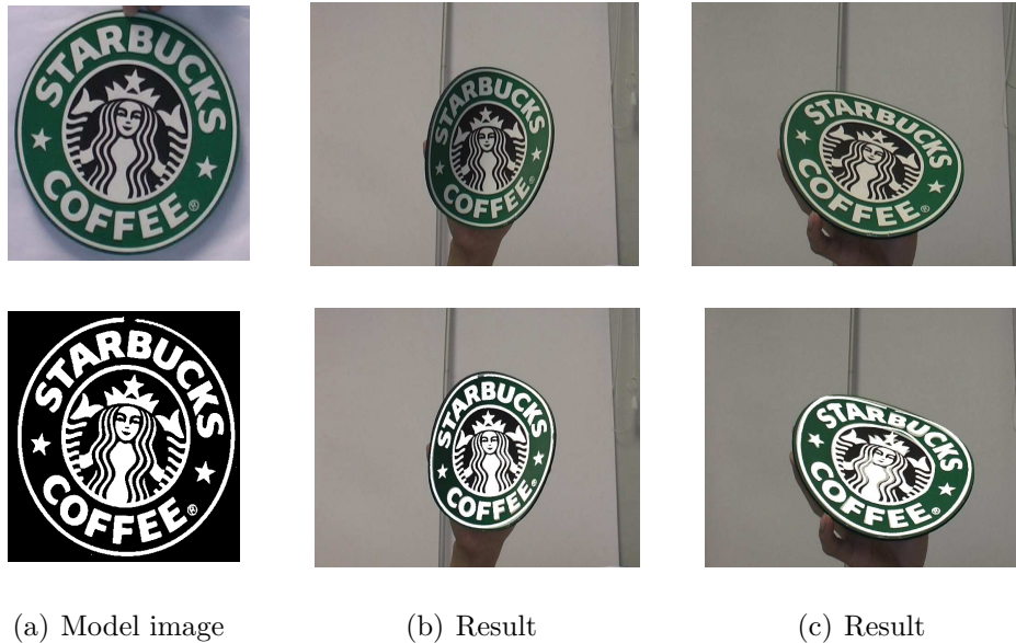
Figure 3.5: A Starbucks pad is used as the deformable object. The model image is shown in (a) the contour of the model image is extracted using a simple gradient and filling operator, which is overlaid on the input image. (b) and (c) show the results. The model contains 120 vertices, and the whole process, including image capturing and rendering, runs around 18 frames per second.
