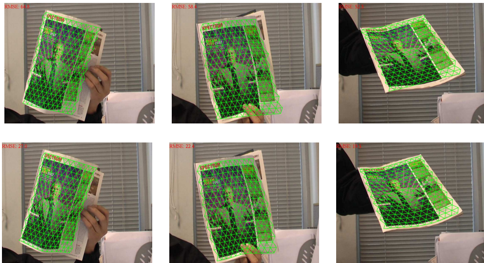
Figure 4.14: Recovering the cover of a magazine in a real-time video with the size of 720 \times 576 . The first row shows the initialization results using feature correspondences only. The second row shows the results with the fusion approach. Moreover, Root Mean Square Error (RMSE) is shown at the left corner in each image.
