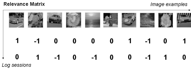
Fig. 2. The relevance matrix for representing the log information of user feedback. Each column of the matrix represents an image example in the image database and each row of the matrix corresponds to a log session in the log database.
