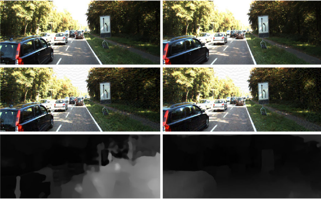
Fig. 11. Examples of AANet disparity results. The defense and test perturbations are both with \epsilon = 10.20 . The images from top to down are: original left and right images, perturbed left and right images, disparity map of the perturbed images generated by the original model, and disparity map generated by SmoothStereoV2 with SoftPlus \beta = 10 . Our disparity map can well reflect the actual physical characteristics while the outputs of the original model are of chaos.
