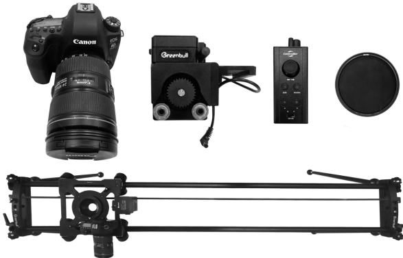
Figure 2: The devices in our mechatronic system. In the top row, from left to right is Canon EOS 6D Mark II, the electric machine (to drive the motion of the camera), the controller (to set the starting and ending points for motion), and an ND filter. We mount the camera and the electric machine on the electric slide rail, as shown in the bottom row.
