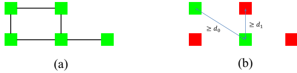
Fig. 6. (a) Via-1 patterns. (b) Layout decomposed to two masks and Via-1 design rules.
