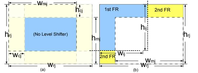
**Fig. 4** (a) No matter how to move the module, dark area can not insert level-shifter, while blank area is Potential White Space(PWS) of  $R_j$  (b) 1st and 2nd Feasible Region of  $FR_{ij}$ .
