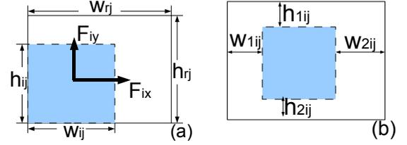
**Fig. 6** In room  $r_j$ , (a) if level-shifter  $ls_i$  prefers to locate in lower-left corner (dark area is prefer region), then  $ls_i$  produces forces  $(F_{ix}, F_{iy})$  to push module  $n_j$  upper and right. (b)  $w_{1ij}, w_{2ij}, h_{1ij}, h_{2ij}$  are defined to calculate forces  $(F_{ix}, F_{iy})$ .
