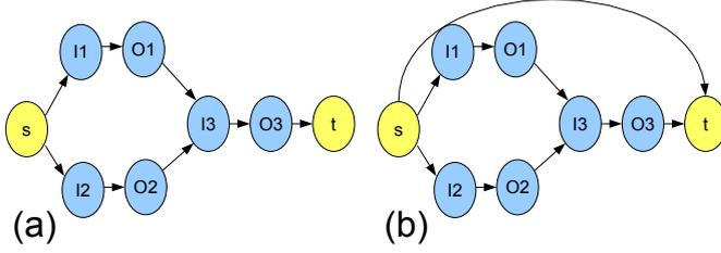
**Fig. 2** (a)  $\bar{G} = \{\bar{V}, \bar{E}\}$ , after adding nodes  $s, t$  and diving nodes  $N_i$  into  $I_i$  and  $O_i$  (b) Transformed  $\bar{G} = \{\bar{V}, \bar{E}\}$  by adding edge  $e(s, t)$  to remove constraint  $\mu_t - \mu_s \leq T_{cycle}$  in equation (2).
