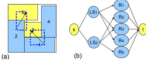
**Fig. 5** (a)  $LS_{13}$  drives from module 1 to module 3 and  $LS_{25}$  drives from module 2 to module 5. (b) Corresponding network graph,  $LS_1$  can be assigned to room 1,3,4, while  $LS_2$  can be assigned to room 2,3,5.
