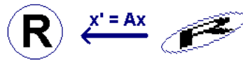
Figure 2.2: This figure shows an example of the elliptical affine region and the normalized region. The transformation matrix A = M^{1/2} projects x to x' such that the eigenvalues of the auto-correlation matrix are equal.
