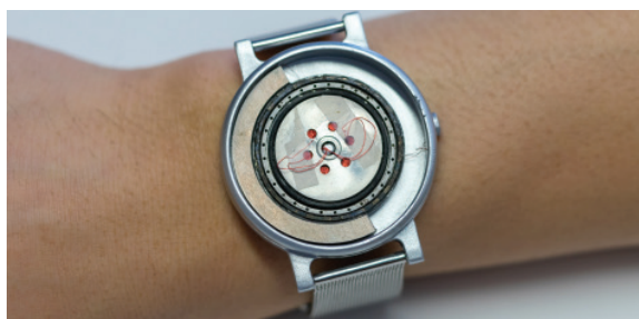
Figure 2 Prototype of the embedded generator
