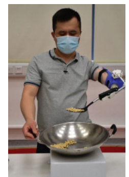
Figure 2.4 Modular prosthetic device with wok tool.
