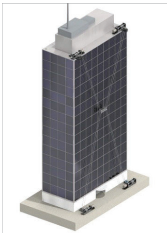
Figure 1.1 Cable-driven parallel robot concept for high-rise façade applications.
