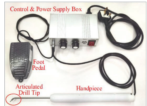
Figure 2. Handheld Articulated Drill System
