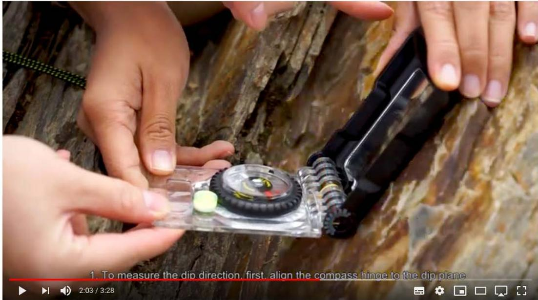
1. To measure the dip direction, first, align the compass hinge to the dip plane
