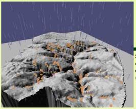
Sediment-laden overland flow is represented by fine cylinder. Where the length of the structure represents velocity, and the inclination of the structure represents the direction of movement. The unit of soil loss is represented by a metaball based on a pixel.
