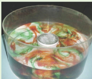
*Weather in a Tank for geophysical fluid dynamics (GFD) experiment using a rotating tank
