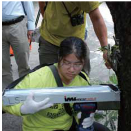
Using different methods to assess the density of a tree in order to determine the extent of internal decay: (left) Mallet method; (centre) Resistograph; and (right) sonic tomograph.
