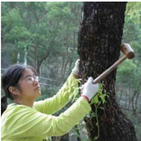
Using different methods to assess the density of a tree in order to determine the extent of internal decay: (left) Mallet method; (centre) Resistograph; and (right) sonic tomograph.
