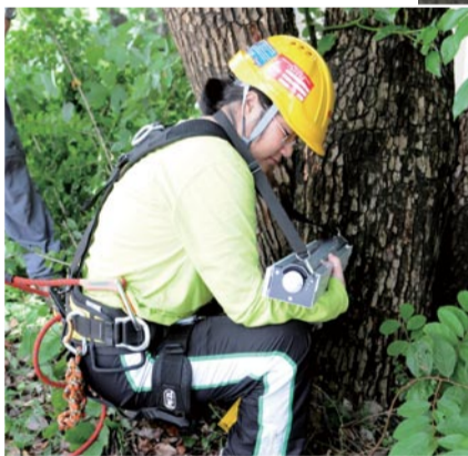
生命科學學院學生伍雪瑩以阻抗圖譜儀檢查樹木 Shirley Ng, a student of the School of Life Sciences, examines a tree with a resistograph
