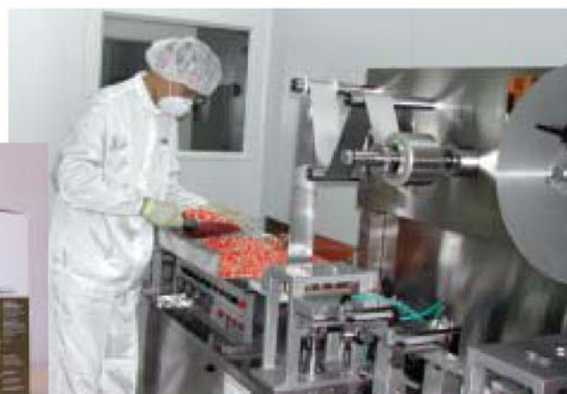
中藥產品下游開發及科研中心的膠囊鋁塑包裝貯存設施 Process Development and Manufacturing Facility for Chinese Medicine: capsules blistered for better storage
