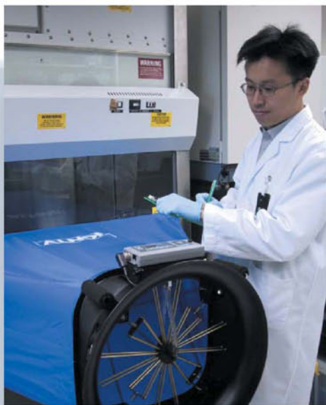
檢查通風系統的性能 Inflow velocity test for an air system
