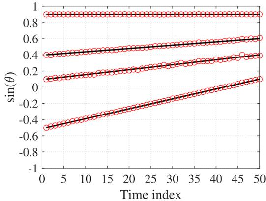
Fig. 6. ss-FRI DOA estimation ( $\circ$ ) with snapshots ( $L = 3$ ) for four moving sources (solid line) with different SNR = 10 dB, 0 dB, 5 dB and 20 dB (in order of DOAs from small to large) respectively for non-uniform array (the array is the same as Fig. 5(c)).
