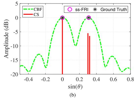
Fig. 7. Single snapshot CS performance in DOA estimation in terms of the discretization of the DOA space. CBF, CS and ss-FRI reconstruction for two equal strength incoherent sources at  $0$  and  $0.31$  with SNR = 20 dB. CBF and CS are (a) on a grid  $[-1 : 0.01 : 1]$ , and (b) on a grid  $[-1 : 0.02 : 1]$ . The ULA has 10 sensors.
