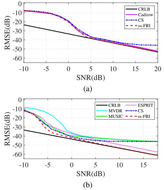
Fig. 11. Comparing the performance curve (averages over 2000 realizations) of Cadzow, MVDR, MUSIC, CS, ESPRIT and ss-FRI DOA estimation with CRLB. There are two equal strength incoherent sources at  $-0.205$  and  $0.505$  with (a)  $L = 1$  and (b)  $L = 10$ . The ULA has 11 sensors.
