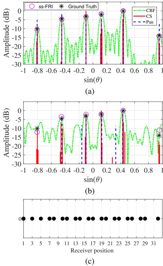
Fig. 4. Single snapshot DOA estimation for uniform and non-uniform array. The sources (\*) are at  $-0.8033, -0.45, -0.1, 0.12, 0.436$  and  $0.953$  with SNR = 10 dB, 15.5 dB, 17 dB, 18 dB, 20 dB, and 6 dB, respectively. Reconstruction of incoherent sources using CBF, Pan's method, CS and ss-FRI DOA estimation (a) for the ULA (b) and for the non-uniform array. (c) The non-uniform array constructed by randomly selecting  $M = 20$  sensors out of a standard ULA with 32 sensors.
