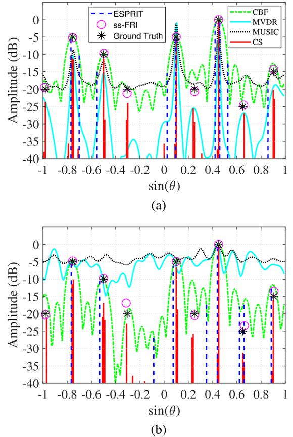
Fig. 3. Multiple snapshot ( $L = 5$ ) DOA estimation for nine sources (\*) at  $-0.98, -0.755, -0.5, -0.305, 0.1, 0.25, 0.45, 0.65,$  and  $0.905$  with SNR = 0 dB, 15 dB, 10 dB, 0 dB, 15 dB, 0 dB, 20 dB,  $-5$  dB, and  $5$  dB, respectively. CBF, MVDR, MUSIC, CS, ESPRIT and ss-FRI DOA estimation for (a) incoherent sources and (b) coherent sources. The ULA has 21 sensors.
