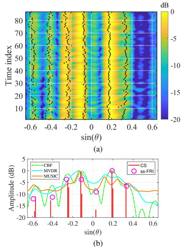
Fig. 13. (a) Single snapshot CBF (background color) and ss-FRI (dots) DOA estimation for frequency  $f = 112$  Hz. (b) Multiple snapshot CBF, MVDR, MUSIC, CS, and ss-FRI DOA estimation for frequency  $f = 112$  Hz.
