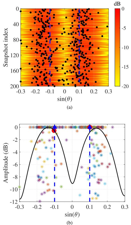
Fig. 9. Comparison of single snapshot and multiple snapshot DOA estimation for two equal strength coherent sources (at 0.1 and  $-0.1$  with  $\text{SNR} = 0$  dB, blue vertical dotted lines) along 200 snapshots. (a) Single snapshot CBF (background color) and ss-FRI DOA estimation (dots). (b) Magnitude distribution of single snapshot ss-FRI DOA estimation (\*), multiple snapshot ss-FRI DOA estimation ( $\circ$ ) and ground truth (arrow). The ULA has 10 sensors.
