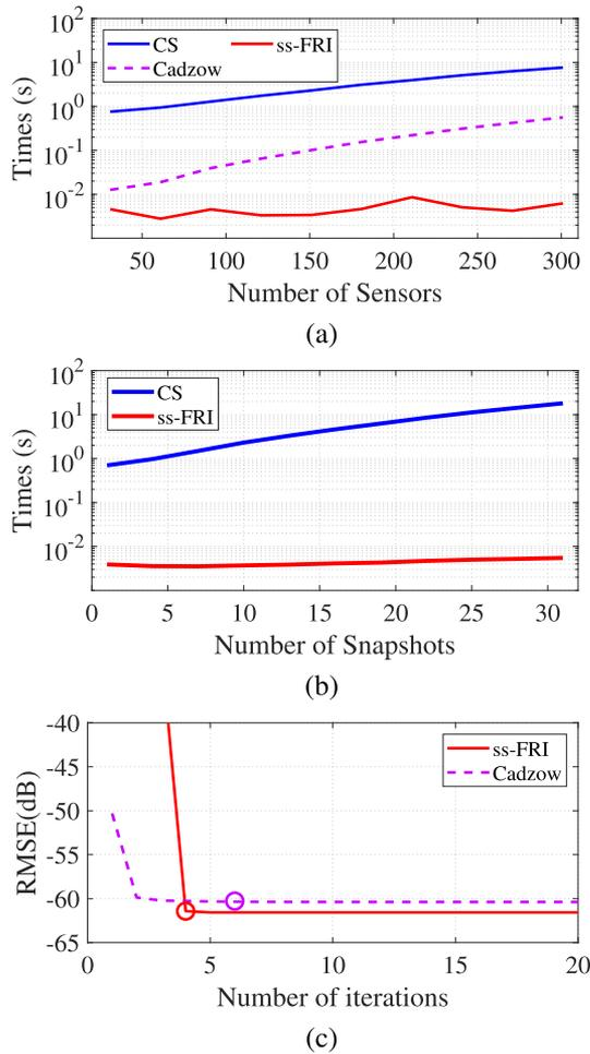
Fig. 12. Comparison of computation time (averages over 500 realizations) for two equal strength incoherent sources with SNR = 15 dB between CS and ss-FRI with (a) different number of sensors  $N$  ( $L = 1$ ) and (b) different number of snapshots  $L$  ( $N = 21$ ). (c) Convergence rate (averages over 2000 realizations) of Cadzow and ss-FRI for two equal strength sources with SNR = 20 dB and 21 sensors. “o” represents the number of iterations to terminate the loop.
