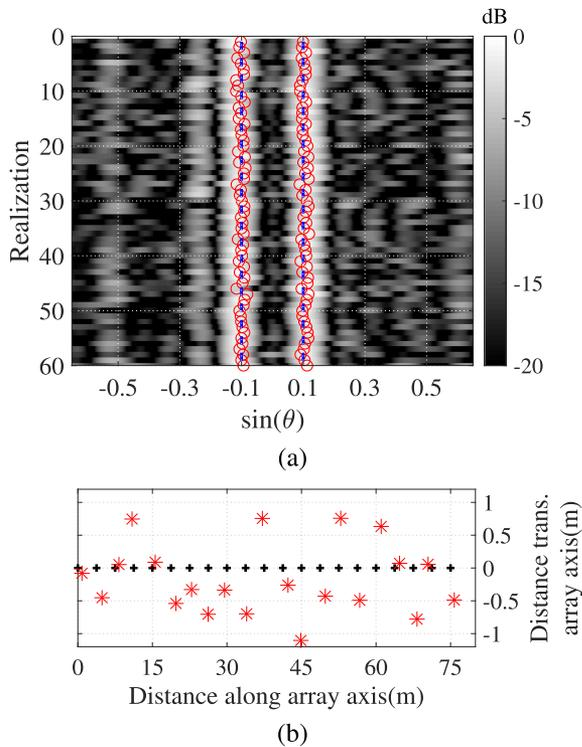
Fig. 8. Single snapshot DOA estimation of two equal strength sources (at 0.1 and  $-0.1$  with  $\text{SNR} = 5$  dB) for 60 realizations with position error. (a) Reconstruction with CBF (background color), ss-FRI DOA estimation ( $\circ$ ) and the true DOAs (the blue vertical dotted line). (b) Top view of the array configuration with position error (“\*”) and no position error (“+”). The ULA has 21 sensors.
