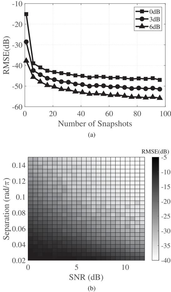
Fig. 10. (a) RMSE (averages over 1000 realizations) for multiple snapshot ss-FRI DOA estimation ( $K = 1$ ) versus number of snapshots with SNR = 0 dB, 3 dB, and 6 dB. (b) RMSE (averages over 1000 realizations) for multiple snapshot ss-FRI DOA estimation versus SNR and Separation between two equal strength incoherent sources with  $L = 5$ . Note that the ULA has 10 sensors.
