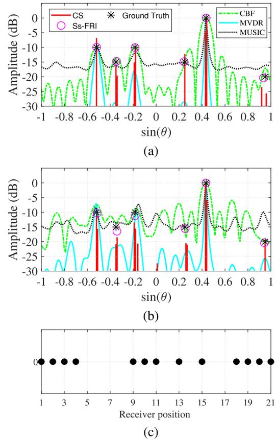
Fig. 5. Multiple snapshot ( $L = 3$ ) DOA estimation for uniform array and non-uniform array. The six sources (\*) are at  $-0.52, -0.35, -0.184, 0.25, 0.436$  and  $0.95$  with SNR = 10 dB, 5 dB, 10 dB, 5 dB, 20 dB, and 0 dB, respectively. Reconstruction of incoherent sources using CBF, MVDR, MUSIC, CS and ss-FRI DOA estimation (a) for the ULA (b) and for non-uniform array. (c) The non-uniform array constructed by randomly selecting  $M = 13$  sensors out of a standard ULA with 21 sensors.
