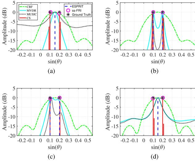
Fig. 2. DOA estimation from  $L$  snapshots for two equal strength sources (\*) at 0.1 and 0.2 with SNR = 20 dB. CBF, MVDR, MUSIC, CS, ESPRIT and ss-FRI DOA estimation for incoherent sources with (a)  $L = 1$ , (b)  $L = 64$ , and (c)  $L = 3$ , and (d) for coherent sources with  $L = 64$ . The ULA has 10 sensors.
