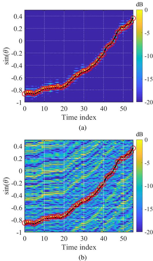
Fig. 14. DOA trajectory estimation (frequency  $f = 1800$  Hz) for CBF (background color), ss-FRI ( $\circ$ ), and GPS (solid line). (a) ULA. (b) Non-uniform array. Note that the non-uniform array constructed by randomly selecting  $M = 12$  sensors out of a standard ULA with 96 sensors.
