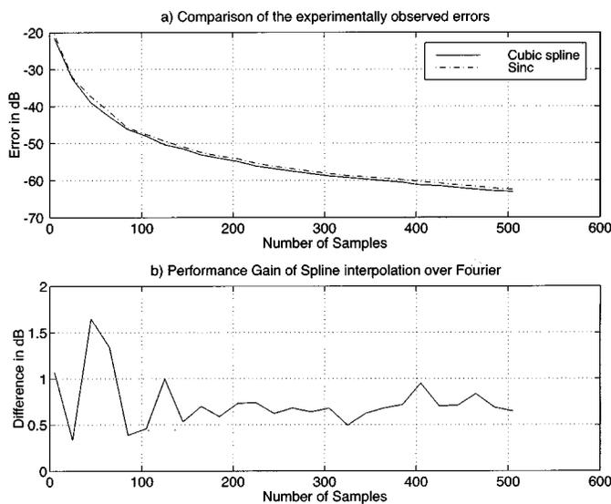
Fig. 3. Comparison of spline and sinc interpolation.
