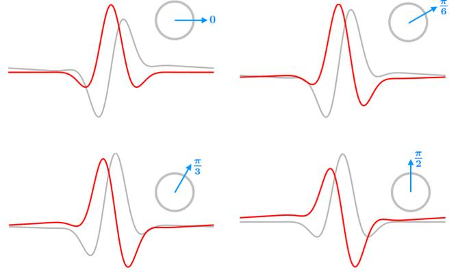
Fig. 2: We plot real (red) and imaginary (grey) parts of pulse  $e^{j\theta_k} \varphi(t)$ ,  $\theta_k = \pi k/6$ ,  $k = 0, \dots, 4$  where  $\varphi$  is chosen to be a modulated Gaussian function (Gabor window) such that the real and imaginary parts form a quadrature pair.
