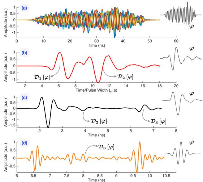
**Fig. 1:** Disparate case studies where the measurements are delayed, amplitude-scaled and distorted versions of the reference pulse  $\varphi$  shown in the inset. (a) Electron laser measurements in Electron Paramagnetic Resonance. (b) Photoacoustic imaging. (c) Ground penetrating radar. (d) Ultra-wide band array.
