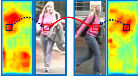
Figure 5. Illustration of bi-directional weighting for patch matching. Patches in red boxes are matched in dense correspondence with the guidance of corresponding saliency scores in dark blue boxes.
