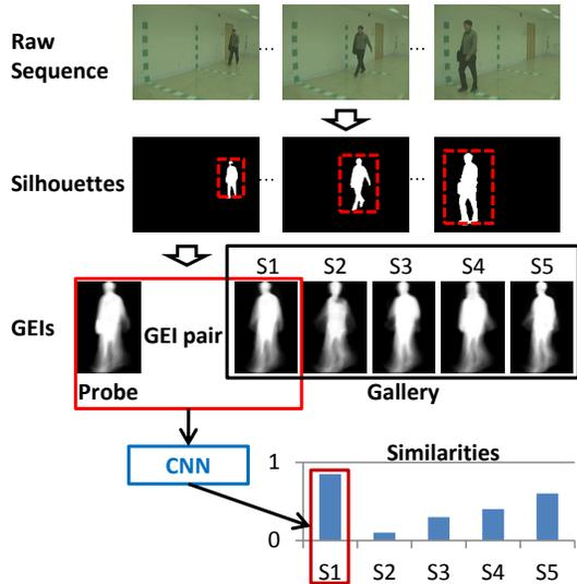
Fig. 3. Pipeline of a typical GEI-based gait recognition method. The probe sample is assigned to S1, which is evaluated as the most similar one.
