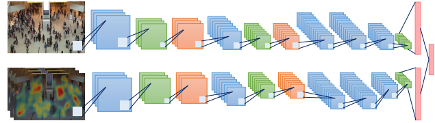
Figure 5. Deep model. The appearance and motion channels are input in two separate branches with the same deep architecture. Both branches consist of multiple layers of convolution (blue), max pooling (green), normalization (orange), and one fully-connected (red). The two branches then fuse together to one fully-connected layers (red).
