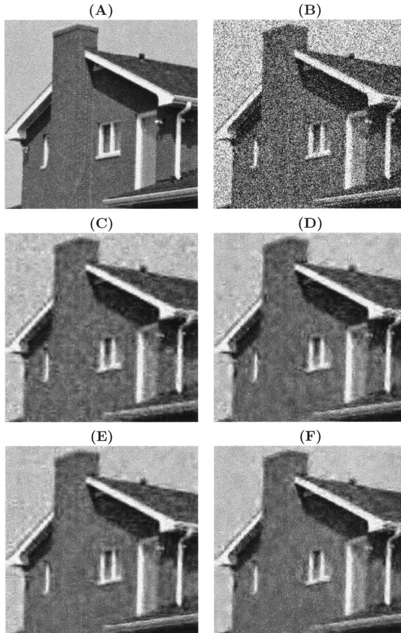
Fig. 12. (a) Part of the noise-free  $256 \times 256$  *House* image. (b) Noisy version of it: PSNR = 18.59 dB. (c) Denoised result using the *BayesShrink*: PSNR = 27.57 dB. (d) Denoised result using the *BiShrink*  $7 \times 7$ : PSNR = 28.19 dB. (e) Denoised result using the *BLS-GSM*  $3 \times 3$ : PSNR = 28.73 dB. (f) Denoised result using our interscale dependent thresholding function (21): PSNR = 28.96 dB.
