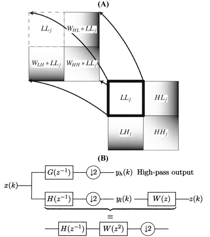
Fig. 7. One way of obtaining the whole parent information out of the lowpass subband: (a) 2-D illustration; (b) 1-D filterbank illustration.
