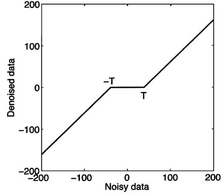
Fig. 2. *Soft-thresholding* function.
