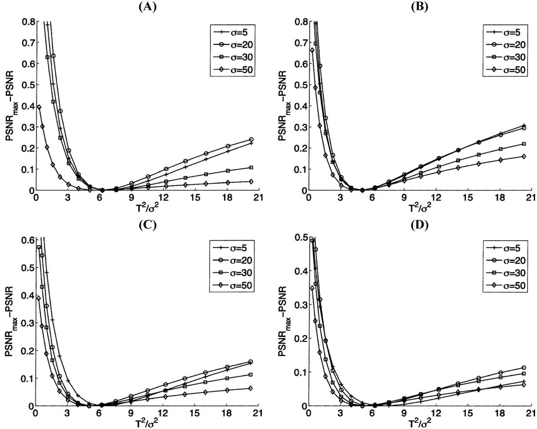
Fig. 5. Sensitivity of our denoising function (14) with respect to variations of  $T$ . (a) *Peppers*  $256 \times 256$ . (b) *MIT*  $256 \times 256$ . (c) *Lena*  $512 \times 512$ . (d) *Boat*  $512 \times 512$ . We can notice that for all images and for the whole range of input PSNR the maximum of the PSNR is reached for  $(T^2/\sigma^2) \simeq 6$ .
