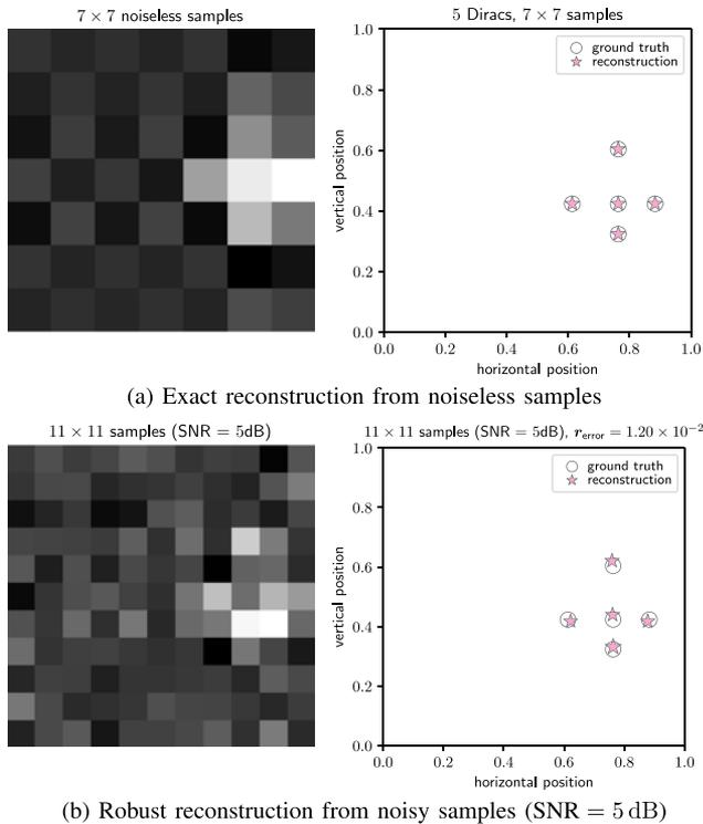
Fig. 7. Reconstruction of 2D Diracs, some of which have common  $x$  or  $y$  coordinates, with the joint estimation (6). (a) The exact reconstruction from the noiseless ideally low-pass filtered samples (sample size:  $7 \times 7$ ). (b) Robust estimation of 2D Diracs from noisy samples (sample size:  $11 \times 11$ , SNR = 5 dB, reconstruction error on the Dirac locations:  $1.2 \times 10^{-2}$ ).
