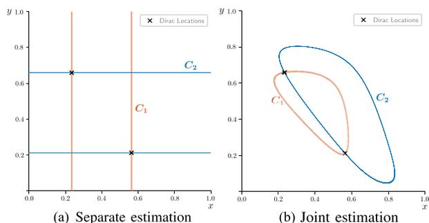
Fig. 2. Joint estimation of 2D Diracs based on curve intersections. The Dirac locations are given by the intersections of two curves  $C_1$  and  $C_2$  (see text in Section II-B2). (a) The zero-crossings of two univariate polynomials specified by two 1D annihilating filters in the separate estimation (Section II-B1). (b) The zero-crossings of two (bivariate) polynomials specified by general shaped 2D annihilating filters in the joint estimation.
