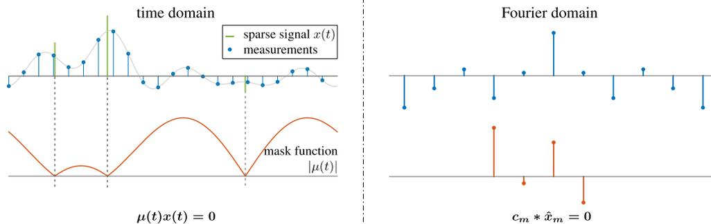
Fig. 1. Sensing sparsity through annihilation: instead of recovering the sparse signal  $x(t)$  directly, the FRI-based approach estimates a smooth function  $\mu(t)$ , which vanishes at the non-zero locations of the sparse signal. The continuous-domain constraint  $\mu(t)x(t) = 0$ , can be equivalently enforced with a discrete convolution equation in Fourier domain:  $c_m * \hat{x}_m = 0$ , where  $c_m$  is known as the “annihilating filter” (see text in Section II-A1 for details).
