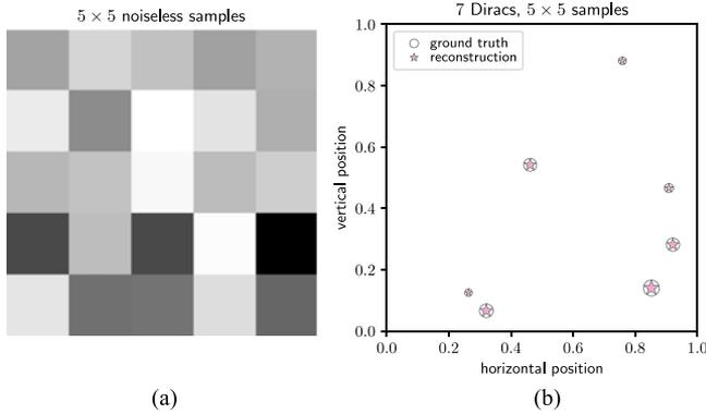
Fig. 5. Exact reconstruction of 7 Diracs on a 2D plane from  $5 \times 5$  ideally low-pass filtered samples. (a) The noiseless ideally low-pass filtered samples. (b) The exact reconstruction with the proposed joint estimation. The joint annihilation approach utilizes the given measurements efficiently. In comparison, the separate annihilation approach (5) fails to reconstruct any Dirac, because it requires a minimum sample size  $8 \times 8$  in this case.
