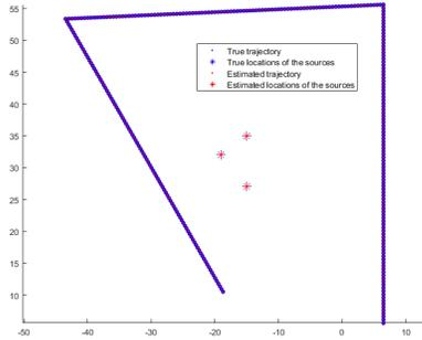
**Fig. 4:** Estimation of the locations of 3 sources and the sampling trajectory composed of 3 linear segments, when the first two segments of the trajectory are known.
