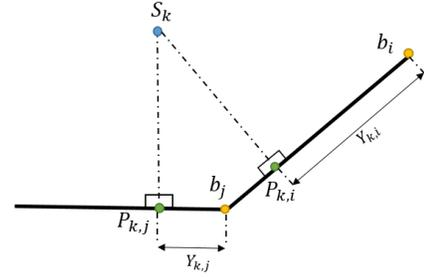
**Fig. 2:** Estimating the location of source  $\mathbf{S}_k$ , using measurements along two different lines  $i$  and  $j$ .
