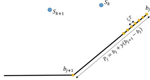
**Fig. 1:** Measurements at discrete time along linear trajectories, of the physical field created by two diffusion sources.
