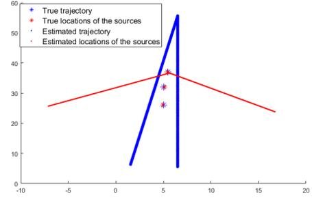
**Fig. 5:** Linearly transformed source locations and trajectory to best fit the true source locations and trajectory respectively, when the samples are corrupted by additive white Gaussian noise of SNR=20dB.
