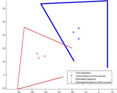
**Fig. 3:** Estimation of the locations of 3 sources and the sampling trajectory composed of 3 linear segments, when the starting point of the trajectory is arbitrary.
