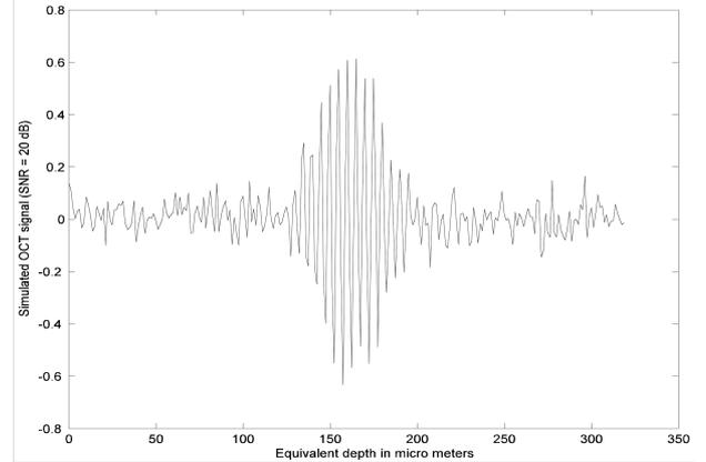
Fig. 1: Example of a simulated OCT signal with a Gaussian coherence function of temporal coherence length 20 $\mu\text{m}$  and corresponding to two layers separated by 2 $\mu\text{m}$  and with SNR=20dB.
