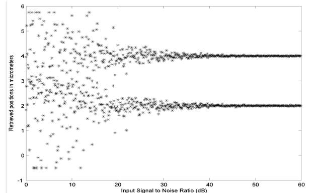
Fig. 2: Retrieved positions of the interfaces as a function of the input noise: for SNR>20dB, the two layers can be separated.
