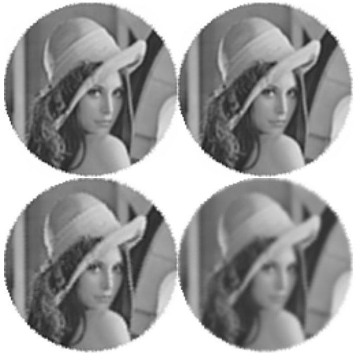
Fig. 1. Compound rotation. Top-left: O-moms \{2, 3, -1, 3\} . Top-right: B-spline \{2, 3, 1, 3\} . Bottom-left: Schaum \{2, 3, -1, 3\} . Bottom-right: Dodgson \{2, 3, 0, 2\} . Dodgson (less order) results in somewhat more blurring than the other cases (more order). Further benefit results from relaxing the interpolation constraint (O-moms, B-spline). The regularity plays no role.
