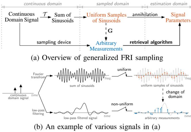
Fig. 3. Any continuous domain signal, which can be represented as a sum of sinusoids by applying a certain transformation  $\mathcal{T}$ , is an FRI signal. The classic FRI framework reconstructs the continuous domain signal from a set of *uniform* samples. Our focus in this paper is on cases where measurements are taken irregularly. We will identify a linear mapping  $\mathbf{G}$  that relates uniform samples to these measurements with a good approximation.
