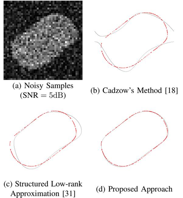
Fig. 10. Visual comparisons of the reconstructed curves with Cadzow's method, structured low-rank approximation [31] and the proposed approach (noise level: 5dB, curve coefficients  $c_{k,l}$  size:  $3 \times 3$ , sample size:  $45 \times 45$ , periods  $\tau_1 = \tau_2 = 1$ ). The solid black line is the reconstructed curve; while the dotted red line is the ground truth.
