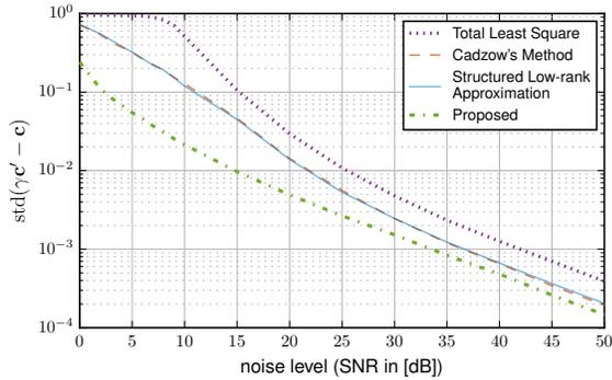
Fig. 9. FRI curve coefficient error against different noise levels (curve coefficients  $c_{k,l}$  size:  $3 \times 3$ , sample size:  $45 \times 45$ , bandwidth  $B_1 = B_2 = 25$ , periods  $\tau_1 = \tau_2 = 1$ ). The results are averaged over 500 independent noise realizations.
