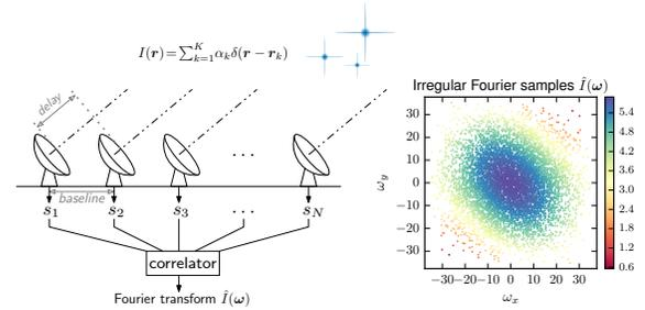
Fig. 1. Schematic diagram of a radio interferometer. The cross-correlations of the received signals at different antennas are related to the Fourier transform of the sky image (see Table I) at certain non-uniform frequencies.
