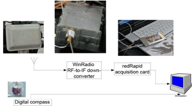
Fig. 10. Schematic diagram of the direction finding receiver.
