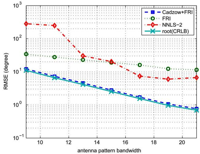
Fig. 7. DOA estimation RMSEs versus the antenna pattern bandwidth for  $N = 512$ ,  $L = 26$  and  $\theta = \{25.208^\circ, 47.7191^\circ\}$ . The SNR is set at  $-5$  dB.
