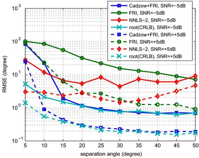
Fig. 8. DOA estimation RMSEs versus the angular separation for  $N = 512$ ,  $L = 26$ ,  $M = 11$  and  $\theta_1 = 25.208^\circ$  while  $\theta_2$  is varied.
