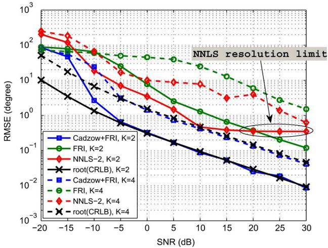
Fig. 9. DOA estimation RMSEs versus SNR for  $N = 512$ ,  $L = 26$ ,  $M = 11$  and  $\theta = \{25.208^\circ, 47.7191^\circ\}$  for  $K = 2$  sources and  $\theta = \{25.208^\circ, 47.7191^\circ, 75.4563^\circ, 105.2431^\circ\}$  for  $K = 4$  sources.
