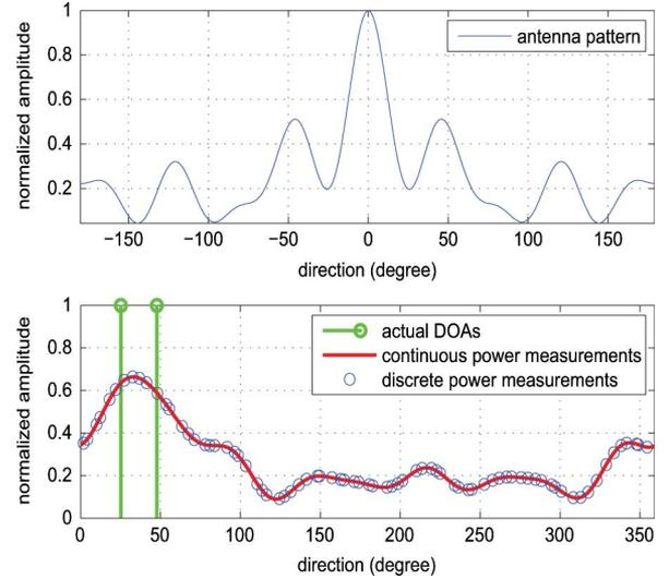
Fig. 1. (a) An example of the realization of antenna pattern simulated according to (2) with  $M = 9$ . (b) The power level versus the direction plotted with the actual DOA locations indicated by ‘—o’.
