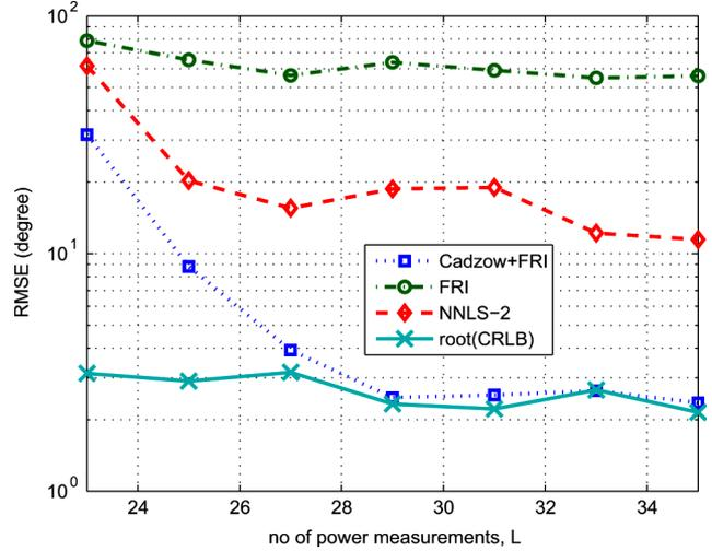
Fig. 6. DOA estimation RMSEs versus the number of power measurements for  $N = 512$  and  $\theta = \{25.208^\circ, 47.7191^\circ\}$ . The antenna pattern is modeled with  $M = 11$  and the SNR is set at  $-10$  dB.
