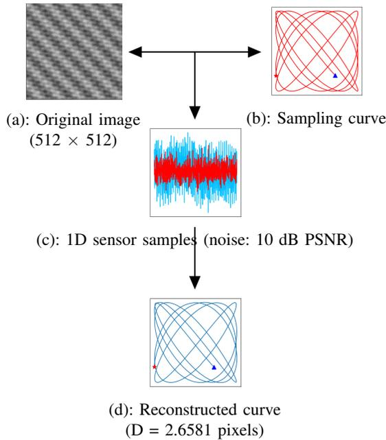
Fig. 5: Trajectory retrieval from 1D sensor measurements sampled from a noisy sinusoidal image (PSNR = 10dB) made up of 10 spatial sinusoids.
