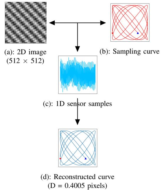
Fig. 4: Trajectory retrieval from 1D sensor measurements sampled from a noiseless sinusoidal image made up of 10 spatial sinusoids.
