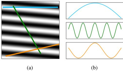
Fig. 2: Sampling an 2D sinusoidal image along different straight lines (a) gives rise to distinct 1D sinusoids (b). For visual intuition, the 2D image is only made up of one spatial sinusoid ( $K = 1$ ).
