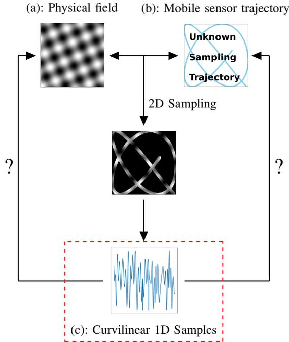
Fig. 1: Our goal is to retrieve the trajectory (b) of the mobile device from the 1D sensor measurements (c) (framed by a red box).
