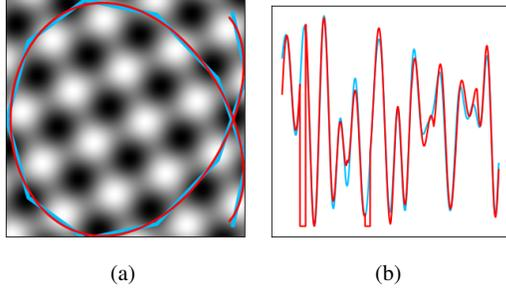
Fig. 3: Piecewise-linear approximation of the curved trajectory. (a) red: ground-truth trajectory, blue: piecewise-linear approximation. (b) red: ground-truth 1D samples, blue: piecewise-linear approximated 1D samples.
