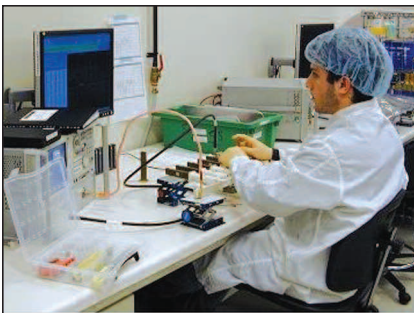
▲ Fig. 3 A tuner uses CAT to tune a six channel MUX.
