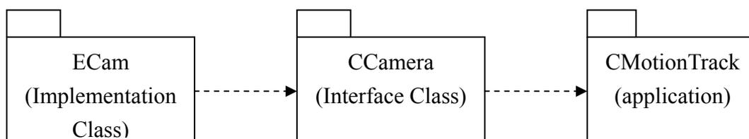
The required asynchronous virtual methods of the CCamera class are implemented in the MotionTrack classes.
