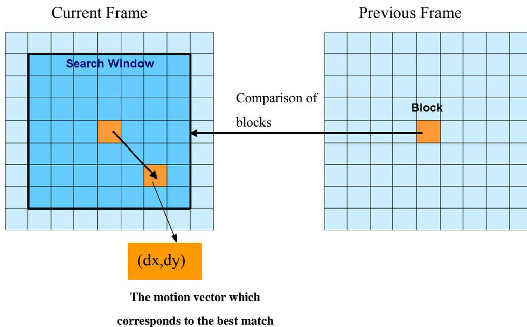
Figure 5.2 Motion tracking: a block is compared against the blocks in the search area in the current frame.
