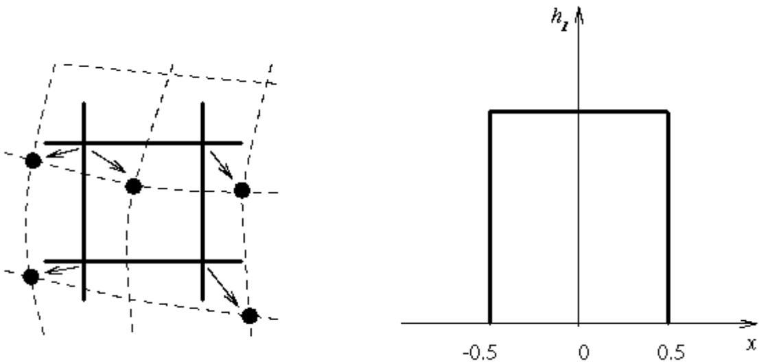
Figure 29: Nearest neighbor interpolation and its brightness function.
