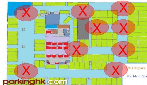
Figure 3.1.2 – Beacons are only deployed on turning point and crossroad
