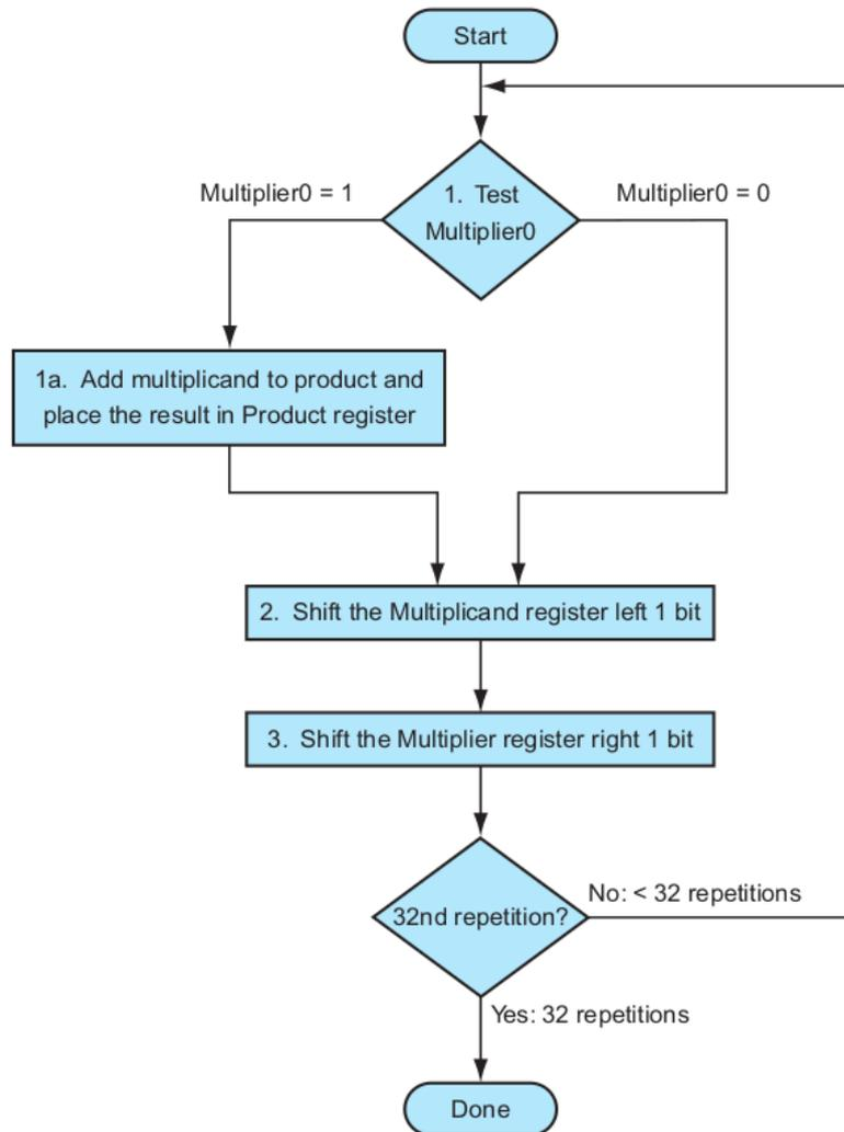
Figure 1: A simple multiplication algorithm.
