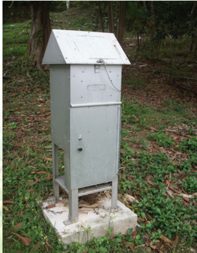
TSP sampler is installed to monitor the roadside dust level. 裝設總懸浮微粒取樣器，監察路邊塵埃水平。
