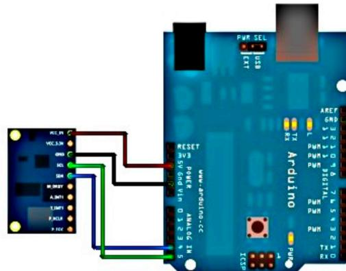
Figure 3: Connection of IMU module
