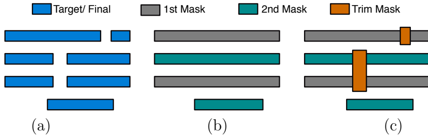
Figure 2.26: Process of LELE-EC type triple patterning lithography (a) Target features; (b) First and second mask patterns; (c) Trim mask, and final decomposition without conflict.
