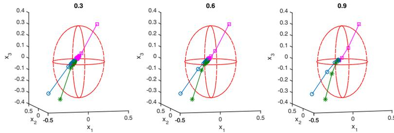
FIGURE 2. Numerical solutions for  $\alpha = 0.3, 0.6$  and  $0.9$  with parameters  $c_1 = 5, c_2 = 6, c_3 = 5, a = 1/2, b = 5$  and the reference ball  $B(0, 1/\sqrt{10})$ . Three orbits are computed by second order F-BDFs with  $h = 0.4$  and  $T = 200$  from the initial values  $(0.3, 0.3, 0.3)^T, (-0.3, 0.3, -0.3)^T$  and  $(-0.3, -0.3, -0.3)^T$ , respectively.
