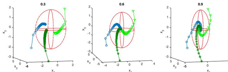
FIGURE 1. Numerical solutions for  $\alpha = 0.3, 0.6$  and  $0.9$  with parameters  $c_1 = 1/4, c_2 = 1, c_3 = 1/4, a = 1/2, b = 1/4$  and the reference ball  $B(0, \sqrt{2})$ . Three orbits are computed by G–L method with  $h = 0.2$  and  $T = 100$  form initial values  $(2, 1, 2)^T, (-2, 3, -2)^T$  and  $(-1, -4, -3)^T$ , respectively.
