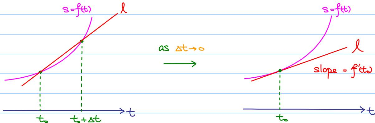
Note : When  $\Delta t \rightarrow 0$  ,  $l$  becomes the tangent line at  $t=t_0$  , so
