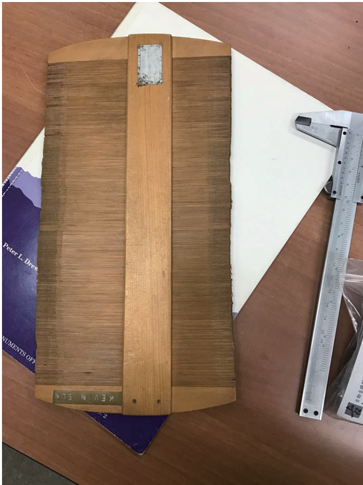
Left: Tool to draw the section of artefact
