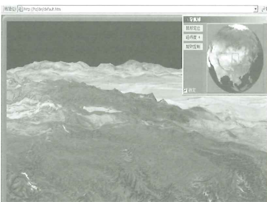
Figure 6. 3D visualization of a part of the earth, f=26.8FPS, n=50125, v=10, p=2.8
